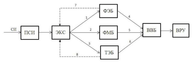
Rice. 1. Diagram of the solar optocoupler device, 1, 2, 3 – optoelectronic circuits, 4, 5, 6 – electrical connecting circuits, 7, 8 – electrical circuits for feedback, VVB – high-voltage unit, FEB – photovoltaic unit,
