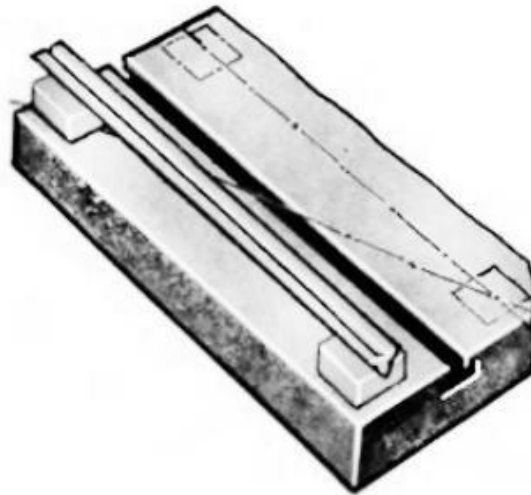
Rice. 3. Scheme for checking the flatness of the working surface of the table
