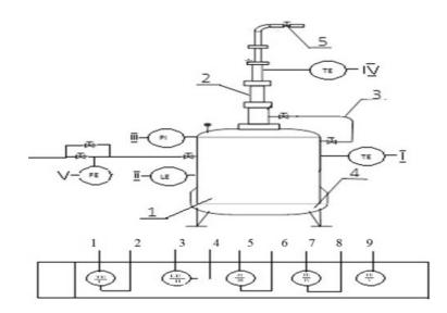
TYe-I tank temperature, RI-III pressure, LE-II level, FE-consumption, TYe-IY column temperature control. is provided by changing the current consumption at the input. The scheme provides automatic adjustment of the ambient temperature by changing the consumption of the heating agent.
